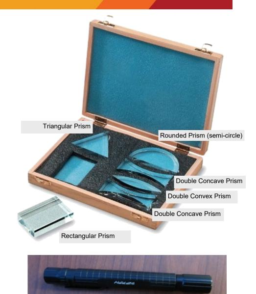
Pen Light (twist the end to focus the light beam)
